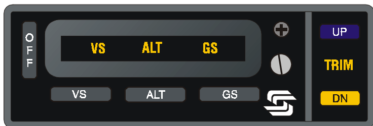
Fig. 3-1. System 60 PSS Programmer/Annunciator
