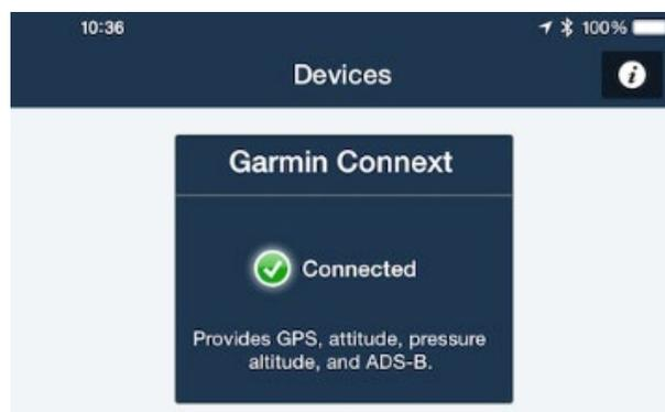
If the Garmin Connex box is not visible, forget the Bluetooth connection using the GNS and then try pairing again.
