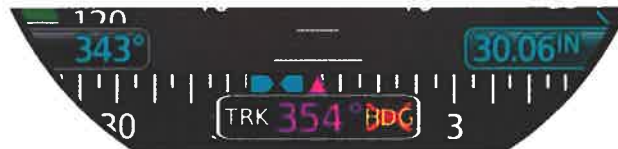
Figure 4- Bottom of the ADI when HDG failed (with GPS)
